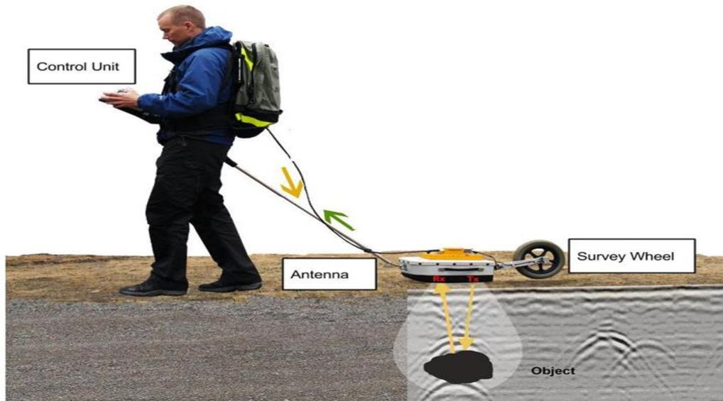
(Figure 1) – Major components of a GPR. (Modified from: <http://www.malags.com/getattachment/Innovation/GPR-Explained/MALA-GPR-principle.jpg>)
